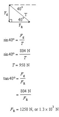
Thus the tension in the wire is 9.6 x  $10^2$  N and the compression in the rod is 1.3 x  $10^3$  N.
