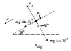
$\vec{F}_{net} = \vec{F}_{down \ slope} + \vec{F}_{f}$   $F_{net} = mg \ \sin 30^{\circ} - \mu_{k} F_{N}$ But  $F_{net} = ma$ , and  $F_{N} = mg \ \cos 30^{\circ}$   $\therefore \ ma = mg \ \sin 30^{\circ} - \mu_{k} \ mg \ \cos 30^{\circ}$ or  $a = g \ \sin 30^{\circ} - \mu_{k} \ g \ \cos 30^{\circ}$   $= \left(9.8 \ \text{m/s}^{2}\right)(0.500) - (0.15)\left(9.8 \ \text{m/s}^{2}\right)(0.866)$
